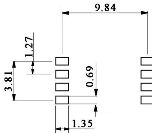
The above footprint layout ensures proper soldering connection interface between the PC board and the sensor PINs when processed by reflow or manual soldering.
